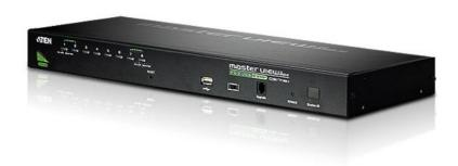
The CS1708A KVM switch is a control unit that allows access to multiple computers from a single PS/2 or USB console (keyboard, mouse, and monitor). A single CS1708A can control up to 8 computers. As many as 31 additional switches can be daisy-chained to each other, so that up to 256 computers can all be controlled from a single keyboard-monitor-mouse console. Additionally, a front panel USB port is available for each computer to access any peripherals connected to it on a one-at-a-time basis.
