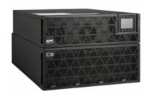
APC Smart-UPS On-Line, 20kVA/20kW, Rack/Tower, 230V/380V...415V, Hard wire 5wire(3P+N+E)+3-wire(1P+N+E), Network Card, W/O rail kit
